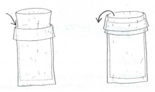
Place the third bag inside the second bag and fold the top down over the first two bags so that cowpeas can be easily poured into the third, inner-most bag.
